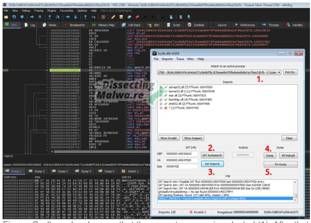
Fire up Scylla and make sure that the correct process is selected (1). After that we'll run the *IAT Autosearch* (2) and *Get Imports* (3) to show them in the textbox above (notice that they significantly differ from the functions imported by the UPX unpacking stub). Finally dump the process to disk (4) and fix the dump (5) to complete the unpacking process. Congratulations to the ones playing along at home, you are now able to manually unpack UPX (and it works for x86 binaries as well).
