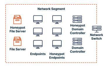
Figure 14-2: Setting up honeypots on a primary network
