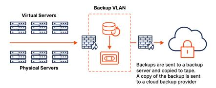
Figure 5-1: A backup network design with offline storage
