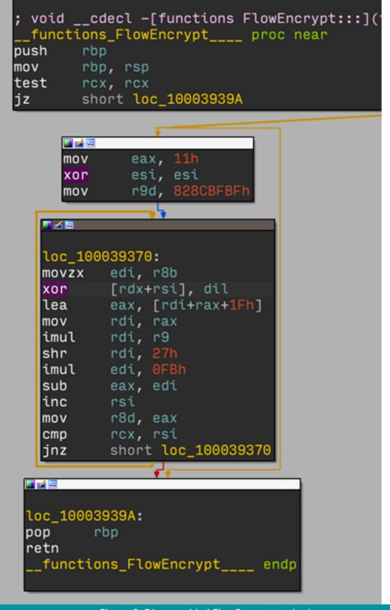
Figure 8. Disassembled FlowEncrypt method
